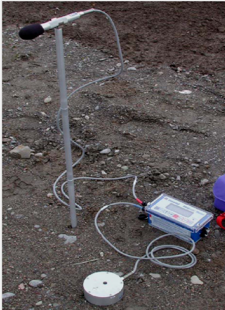
Figure 1 Installing the Minimate Blaster.
